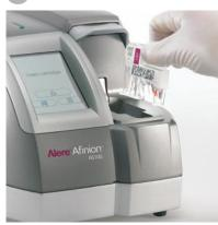
Place the cartridge into the analyzer. The result is displayed within minutes.
