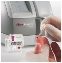
Draw a small volume of sample into the sampling device
