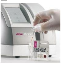
Insert the sampling device into the test cartridge
