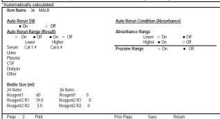
The calibrator (Standard #) values are found in the Quality Control Certificate (SIN212.QC). Calibrator values on Page 1 should be entered in ascending order, i.e. the lowest value first. The analyser will automatically calculate and enter the correct measuring ranges on item pages 3and 4 providing the Autofill button is pressed after typing the value for calibrator 6 on page 1. View Item parameter pages 3 and 4 to ensure correct value entry.
