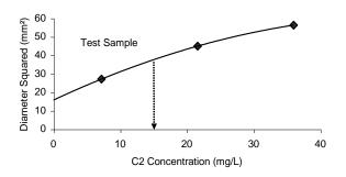
An unknown sample, applied neat as recommended, gave a 6.1mm ring on this plate. From the above curve, this corresponds to a C2 concentration of 14.9mg/L.
