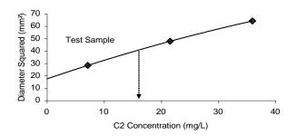
An unknown sample, applied neat as recommended, gave a 6.3mm diameter ring on this plate. From the above curve, this corresponds to a C2 concentration of 16.1 mg/L.
